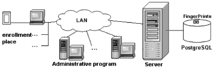
Fig. 2. The structure of the system.
