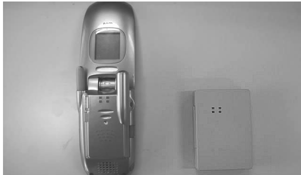
Fig. 5. RFID mobile phone prototype and active RFID
