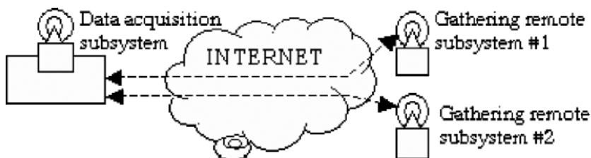
Fig. 2. Remote subsystem communication with GSM GPRS
